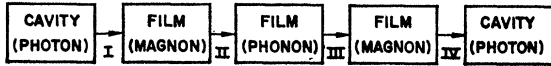
FIG. 1. Diagram of energy flow between the electromagnetic cavity mode, the spin-wave modes in the film, and the acoustic waves in the film.
